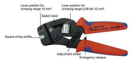
Adjustment of crimp force is possible by actuating the adjustment wheel (see paragr. "Adjustment of crimp force"). The tool ratchet has detents that are audible as "clicks" to close the tool completely, the ratchet automatically releases on last "click", i.e. only after full completion of crimp (forced locking system). To avoid the dies and ferrules being damaged in case of miscrimping, the tool can be emergency released.
