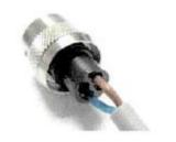
7. Insert contacts into cavaties A & C of the connector
