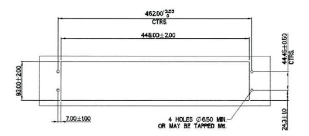
If fitting to a 19" rack that does not support all IEC 60297 fixing holes it may be necessary to use additional mounting plates.
