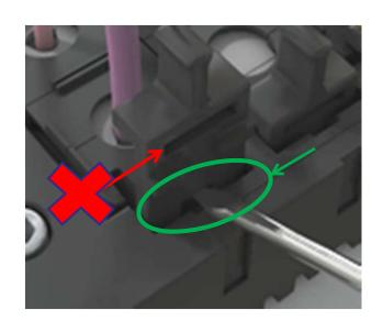
Do **NOT** insert the screwdriver into the large top slot. This can cause the side clip to come out
