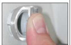
Position the disassembly tool over the latch and push to unlock.
