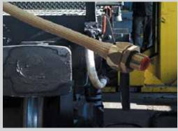
Material: Counter nut, body, clamping ring and ferrule are nickel plated brass with exception of size 3/8" till 1" where the ferrule is from galvanised steel. Inserts are made from PA6 (red for ISO metric, blue for Pg and white for NPT). Temperature: -45 °C till +105 °C continuous (cable-hosefittings till +300 °C on request). Protection class: IP 40. Colour: Metal.
