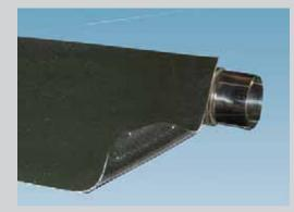
particles of molten splash. **Weight material:** 2,4 Kg/m2 **Temperature:** -55 °C till +260 °C continuous. Under flame till +800 °C for approx. 20 minutes. Radiation heat till +800 °C for approx. 20 minutes. Limited molten metal splash till +1640 °C for 15-30 seconds. **Colour:** Green.
