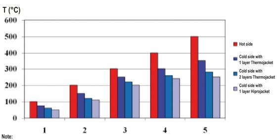
Above mentioned values are based on respectively Hiprojacket Aero and Thermojacket S (saturated) with the heat source at the inside of the sleeving. For additional information on specific conditions, please contact your Anamet representative.
