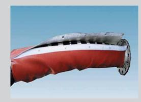
**Cover specifications:** Iron-oxide silicon rubber, excellent oil resistant, halogen-free, good short term flame protection, good temperature reduction, withstands molten splash. Hiproblanket Wrap H-TB enables a finished assembly to be certified to MIL-I-24244, ASTM E84.84A, ASTM E162. **Weight material:** 3,26 Kg/m2
