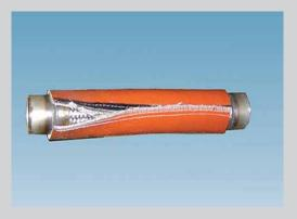
oil resistant, halogen-free, good short term flame protection, good temperature reduction, withstands molten splash. Hiproblanket Wrap H enables a finished assembly to be certified to MIL-I-24244, ASTM E84.84A, ASTM E162. **Weight material:** 3,26 Kg/m2
