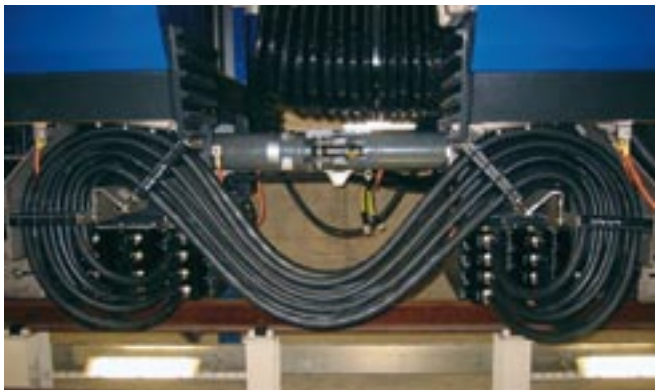
Inter-car Jumper Assembly
