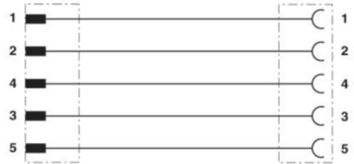
Contact assignment M12-plug and M12-jack
