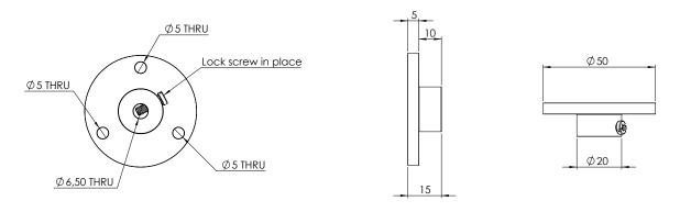
For Ø15mm, Ø22mm or Ø32mm sensor element, cast steel, bolt fitting only, no counter flange
