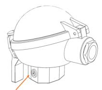
Grounding screw outside of connection head
