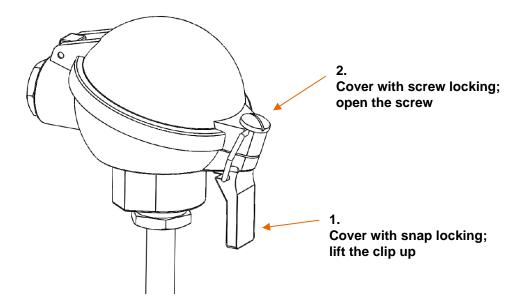
After releasing the locking, lift the cover up.
