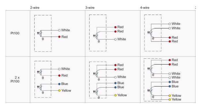
Image below: These are the connection colors of Pt100 resistor connections, according to standard EN 60751.
