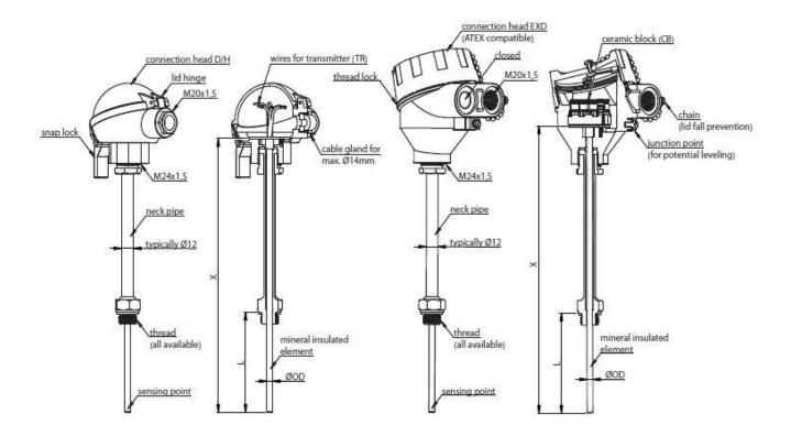
Neck pipe length can be manufactured according to customer specification, e.g. to match the process isolation thickness.
