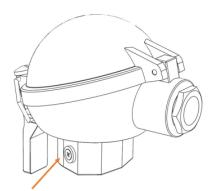
Grounding screw outside of connection head
