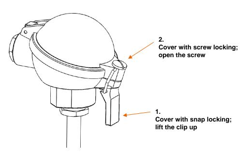
After releasing the locking, lift the cover up.
