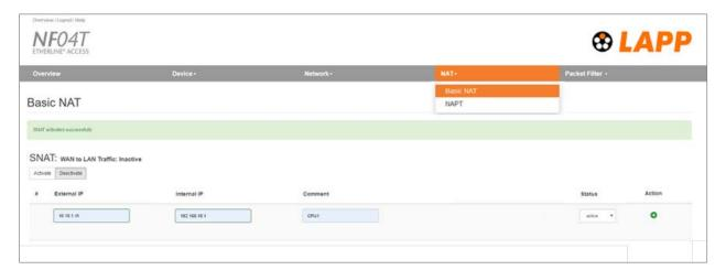
The "External IP" is the IP address under which the network participant of the machine becomes visible in the production network (WAN). The "Internal IP" is the IP address of the network participant in the machine (LAN). Any text can be entered as a comment.
