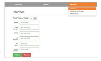
Optionally, the WAN-IP settings, the DNS server, and the standard gateway can also be acquired per DHCP.
