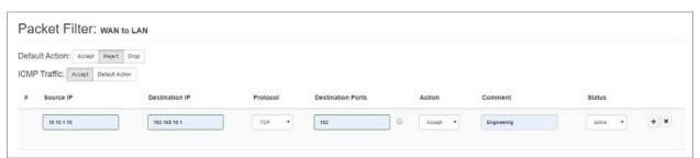
**Source IP** indicates the IP address of the active device in the production network (WAN). **Destination IP** the addressed device in the machine network (LAN).
