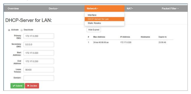
**Primary/Secondary DNS:** DNS server in the LAN for the assignment of the device name, after the ETHERLINE® ACCESS NF04T DHCP server has assigned the IP address to the device.
