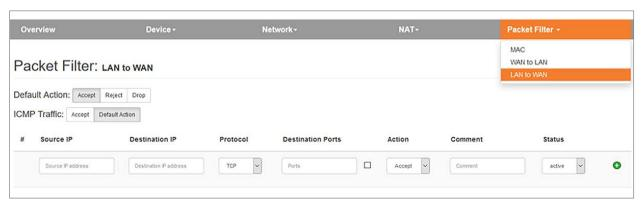
In the "LAN to WAN" packet filter, the communication of devices in LAN with devices in the production network (WAN) can be completely prohibited or be blocked or allowed for particular devices.
