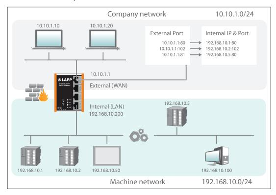
In the following example, the website (Port 80) of the CPU with the IP 192.168.10.5 via WAN can be reached through access to the ETHERLINE® ACCESS NF04T -own IP address 10.10.1.1 with Port 81.
