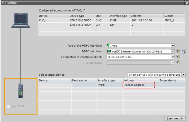
Click on "Access Address" and enter the WAN IP address specified for the device (CPU) in the ETHERLINE® ACCESS NF04T in Basic NAT. Confirm the entry by clicking on the window. An attempt is now made to establish a connection using the entered IP address.
