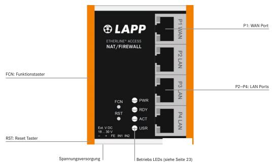
A reset to factory settings can be initiated with the function button (FCN) (see ch. 12). The reset button (RST) initiates a restart of the ETHERLINE® ACCESS NF04T.
