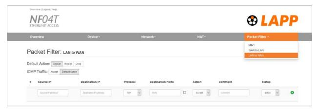
In the "LAN to WAN" packet filter, the communication of devices in LAN with devices in the production network (WAN) or into the Internet is completely prohibited or is blocked or allowed for particular devices.
