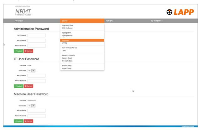
In addition to the "admin" user, which has unlimited access rights, ETHERLINE® ACCESS NF04T supports two more users with limited access rights: "it-user" and "machine-user"
