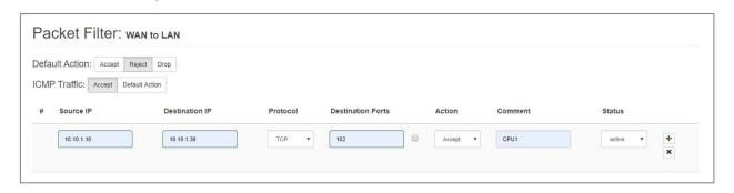
Source IP indicates the IP address of the active device in the production network (WAN).
