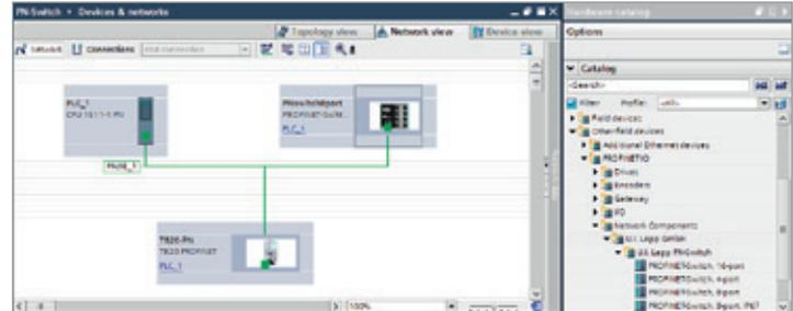
By calling up the object properties, you must assign the PROFINET switch a unique PROFINET name and check the IP address for plausibility in the project.
