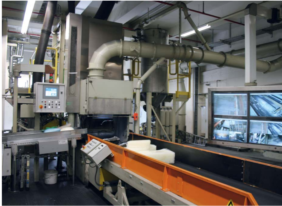
Feeding stage for the internal mixer: The rubber balls are transported here.
