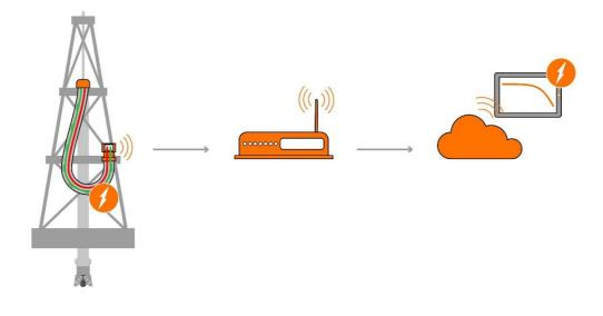
The Smart Service Loop from LAPP uses the changes in the sensor values to calculate when it is time to replace the cable
