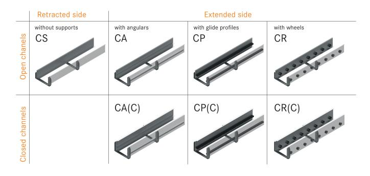
Steel closed channels can be used (on the extended side of the travel distance only) to prevent possible lifting of the chain. Suggested for travel distances LS >40 -50m.
