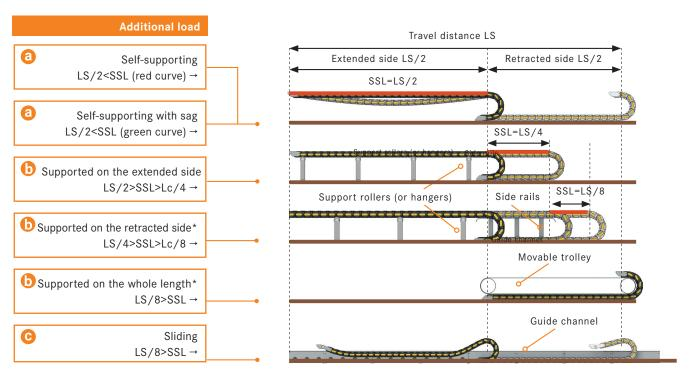
The chain section that is not possible to support is highlighted in red. The combination of additional load and self-supporting length must remain lower than the self-supporting curve of the diagram.
