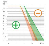
A cable chain can also be used outside its self-supporting area, accepting that the suspended portion of the chain works with a sag. Please also note that cable chains with a sag must be operated with lower speed and acceleration. In addition, the lifetime will be reduced.
