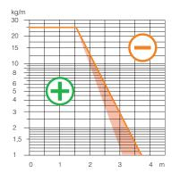
The curve in the self-supporting diagram (orange line) represents the free deviation length of the cable chain (self-supporting length SL) that nullifies the cable chain's pre-set with a certain additional load. The light orange area on the left side (the descending line) of the curve takes into account the fact that, for equal sidebands, a wider cable chain corresponds with a bigger weight and therefore a lower capacity to support the additional load of the utilities.
