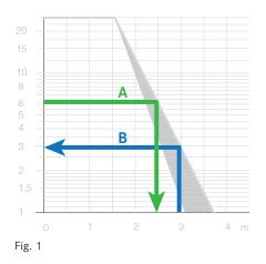
Looking at the diagram (Fig.2), and working in the way "B", the green line level is fixed (because the additional load is determined). Viceversa, the vertical blue line moves to the right increasing the travel distance. When the maximum self-supporting length is exceeded, a configuration has to be chosen that supports the chain in a better way. Generally there are no limitations in the number of support rollers.
