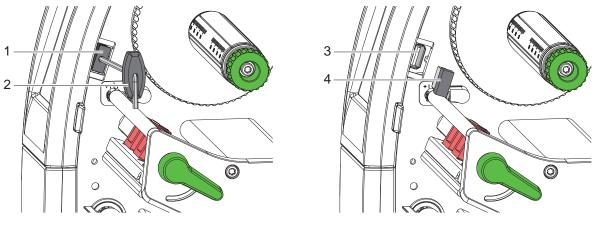
Figure 6 Installing the Wi-Fi stick
