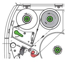
Figure 22 Transfer ribbon feed path
