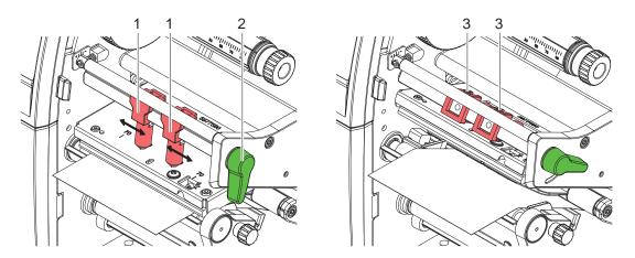
Figure 19 Setting the head locking system - devices with centered media guiding
