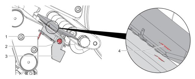
Figure 24 Cleaning the label sensor
