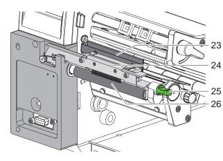
Figure 4 Separator on SQUIX 4MT
