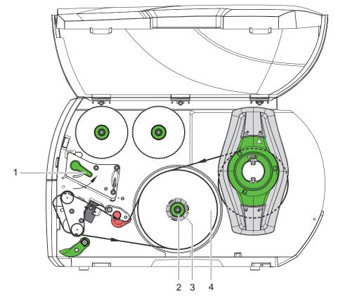
Figure 15 Removing the wound roll
