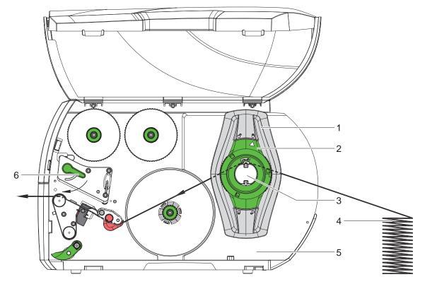
Figure 17 Feed path of fanfold media
