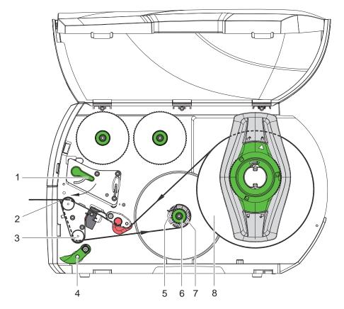
Figure 16 Guidance of the material in peel-off mode
