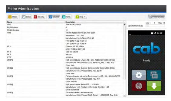
Figure 9 "Devices" tab on the printer web interface
