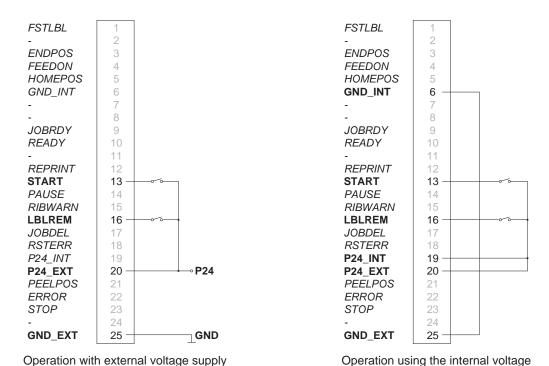
Figure 29 External circuit for peeling-off on demand without present sensor with two signals
