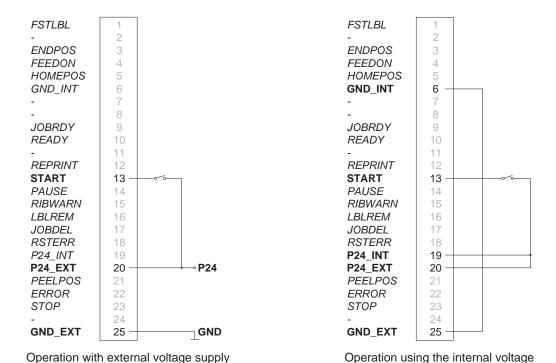
Figure 28 External circuit for peeling-off on demand with Present Sensor PS800 / PS900 / PS1000
