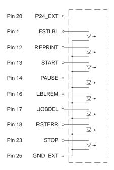
Figure 26 Connecting inputs
