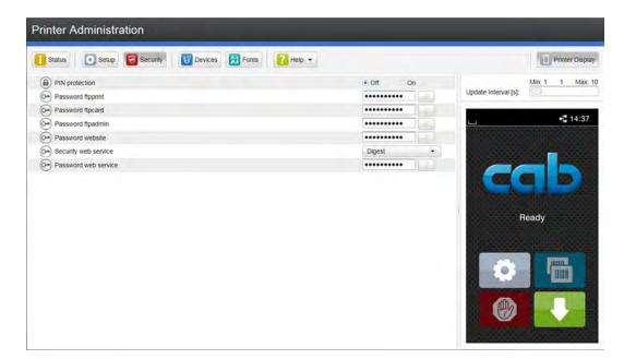
Figure 8 "Security" tab on the printer web interface
