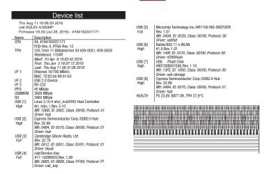
Figure 14 Device list Parameters marked *italic* are only printed when the service key is inserted
