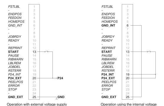
Figure 31 External circuit for peeling-off on demand without present sensor with switching signal START
