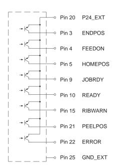
Figure 27 Connecting outputs
