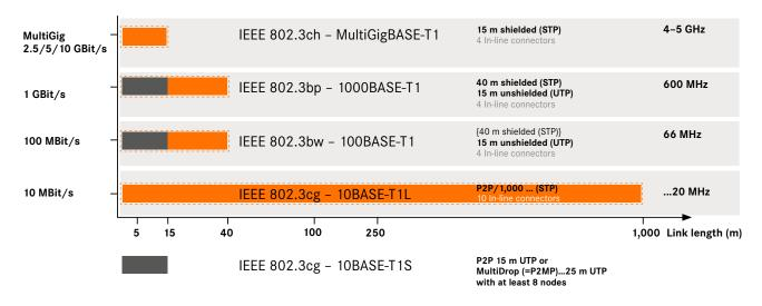
Figure: Overview of the IEEE protocol standards for Single Pair Ethernet
