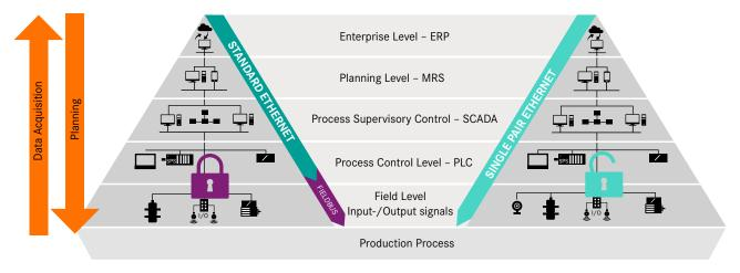
Figure: The change in the industrial network due to Single Pair Ethernet
