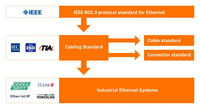
Figure: Overview of standardisation process for Single Pair Ethernet
