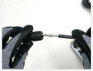
Insert the crimped pin into the connector.
