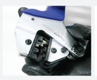
**STEP 5**Partially close the tool, making sure terminal is held in place.
