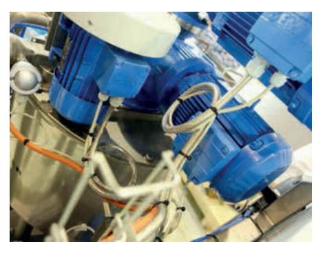
Loops along the cables trap dirt and are tough to clean, so they should be avoided in food production.
