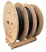
The **multi-chamber drum** can be used for stranding at your construction site. Typically, a material with the same length (e.g.  $3 \times 500$  m) is wound on to this drum. For large drums with a flange diameter of 160 cm or more, free transport racks will be provided for secure transportation and easy handling.
