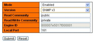
Figure 115 Enable SNMP Protocol and Select SNMP Version
