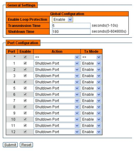
Figure 172 Enable the Loop Detect Function of the Port
