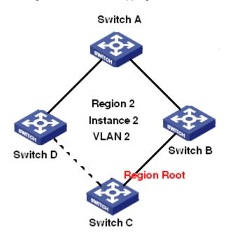
Figure 234 VLAN2 Mapping to Instance 2
