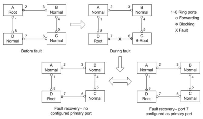
Figure 216 DRP-IEC62439 Link Fault
