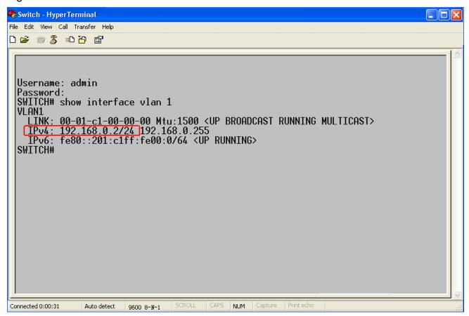
Figure 28 Displaying IP Address
