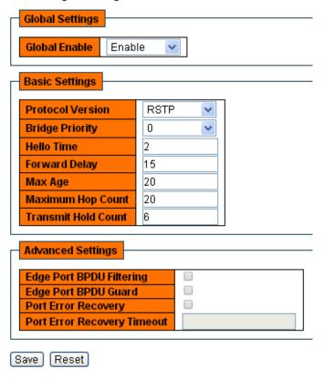
Figure 227 Setting Time Parameters of the Network Bridge
