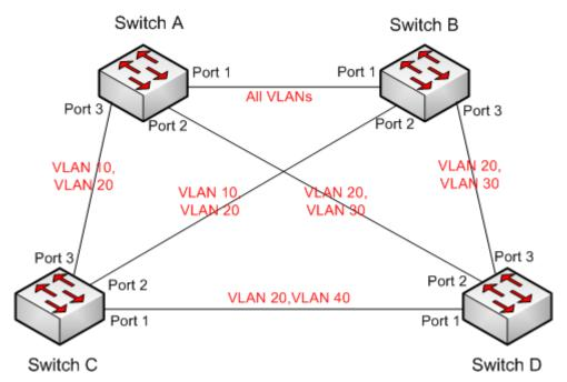
Figure 245 MSTP Typical Configuration Example
