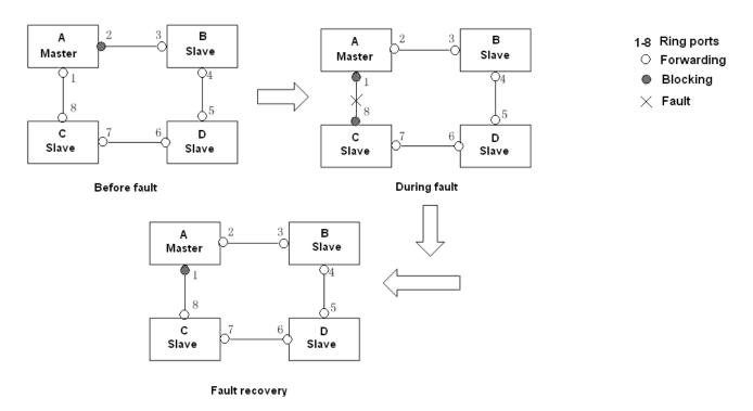
Figure 208 DT-Ring Link Fault
