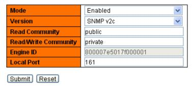
Figure 111 Enable SNMP Protocol and Select SNMP Version
