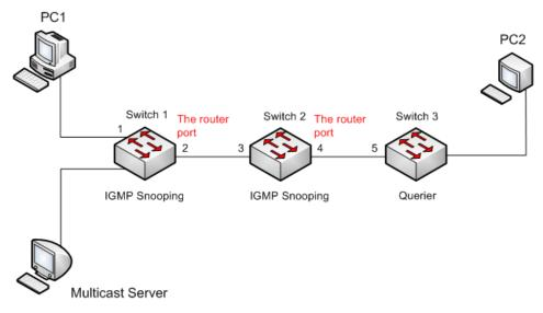
Figure 182 IGMP Snooping Application Example
