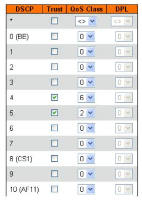
Figure 70 Configure DSCP-based Queue Mapping Mode
