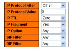
Figure 159 Configure IPv4 Frame Parameters
