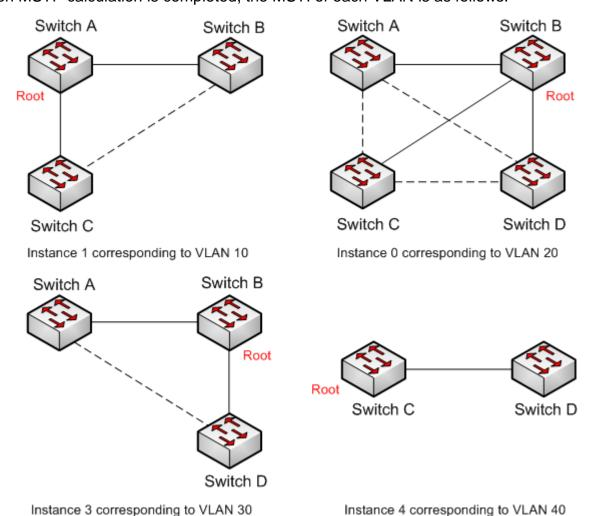
······Blocked link through MSTP calculation
