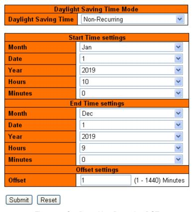
Figure 50 Configure Non-Recurring DST
