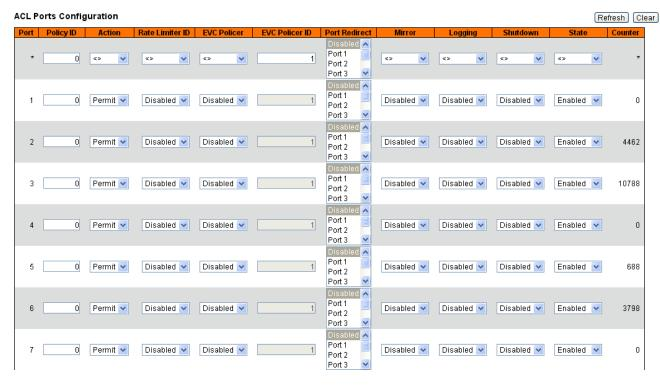
Figure 153 Configure ACL Ports
