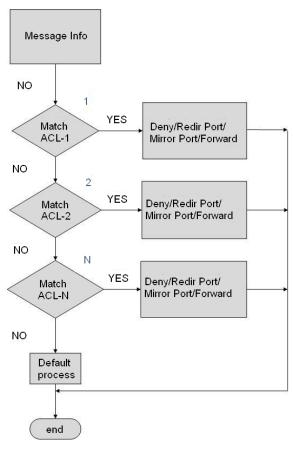
Figure 152 ACL Processing Flowchart
