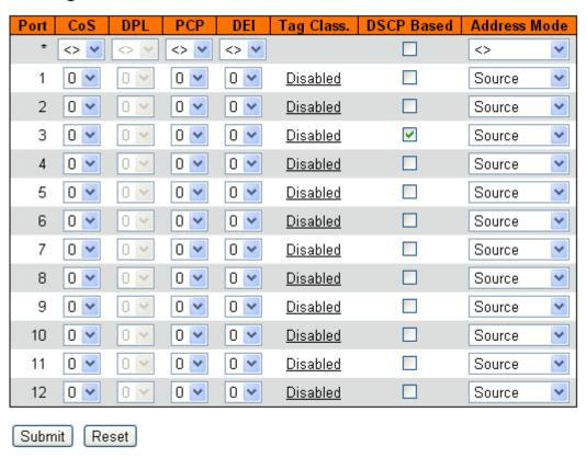
Figure 68 Enable DSCP-based Queue Mapping Mode
