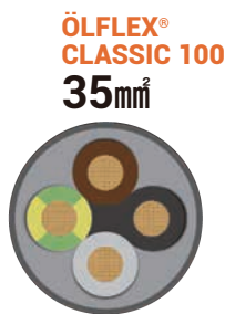
ÖLFLEX® CLASSIC 100 35mm 2 4G35 (35mm 2 -4C) 許容電流:135A 耐電圧:4,000V
