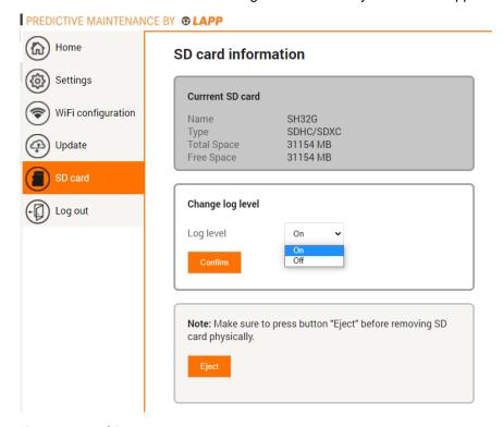
If there is an SD card in the unit, the cable readings are automatically stored there.
