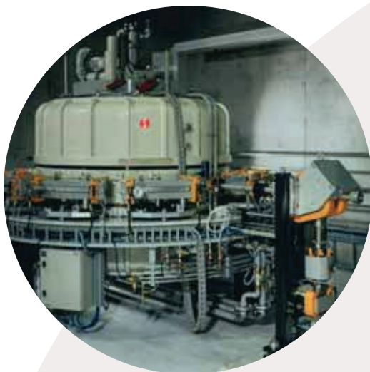
Electron-beam accelerator to cross-link the new LAPP KABEL TRAIN - cables
