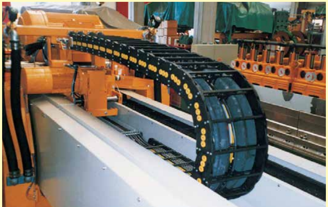
Nylon chain, type 310, in a self-supporting state.
