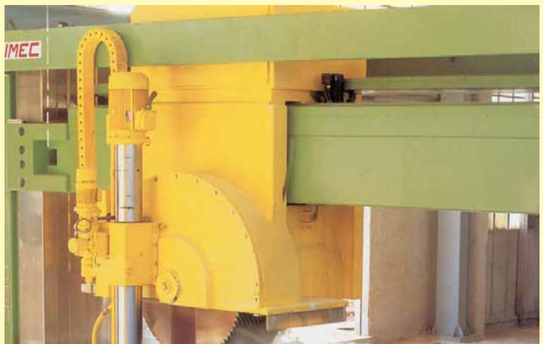
700 yellow nylon chain with the pins in black.
