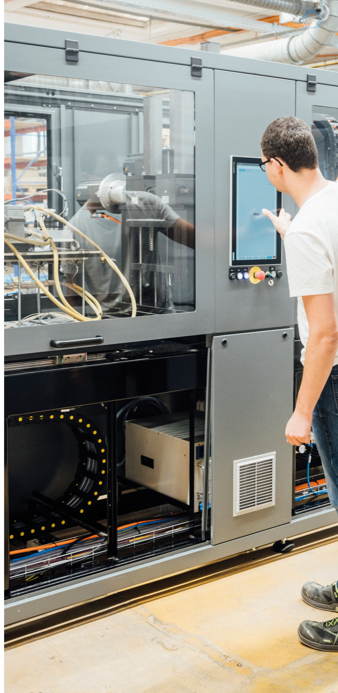
The pullCUBE offers unique safety due to its closed system as well as easy operation through a touch control panel
