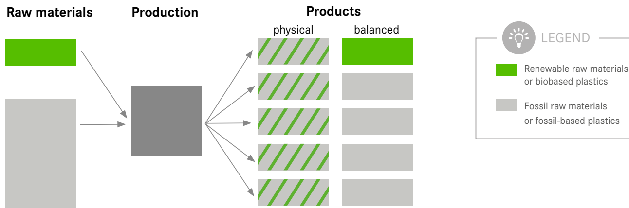
Figure 5: Calculation of the bio-content in partially biobased plastics 12
