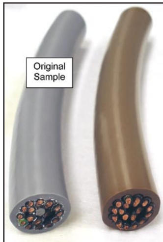
Fig. 5: Discoloring – Caused during the exposure of the PVC to oil or other chemicals due to the diffusion of the plasticizers along with colorant from the insulation and jacket.
