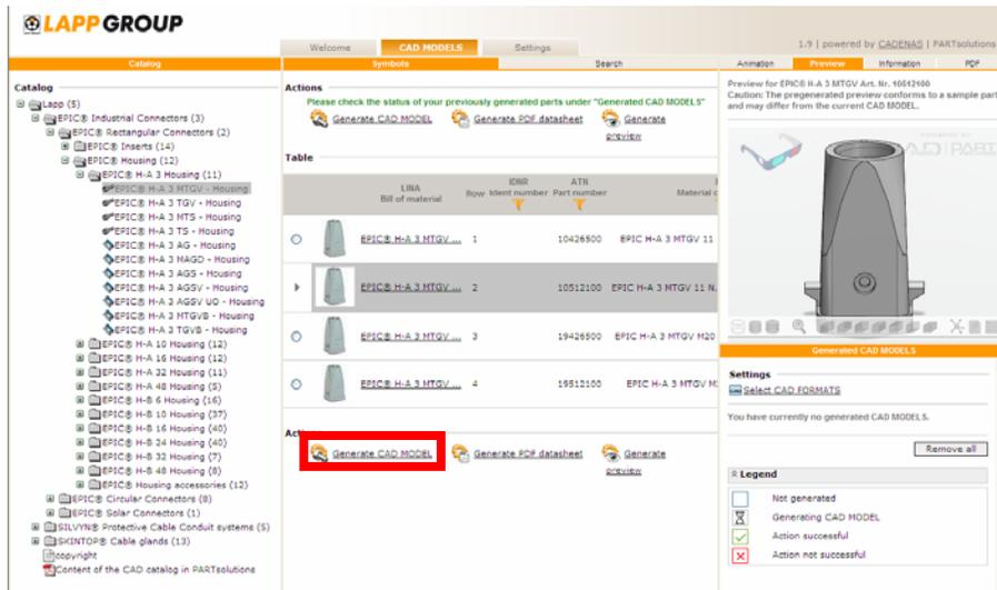
The CAD models can be exported onto your own CAD system, downloaded or emailed. After each formatting criteria selection, make sure to click the “double arrow” so that it is captured in the system.
