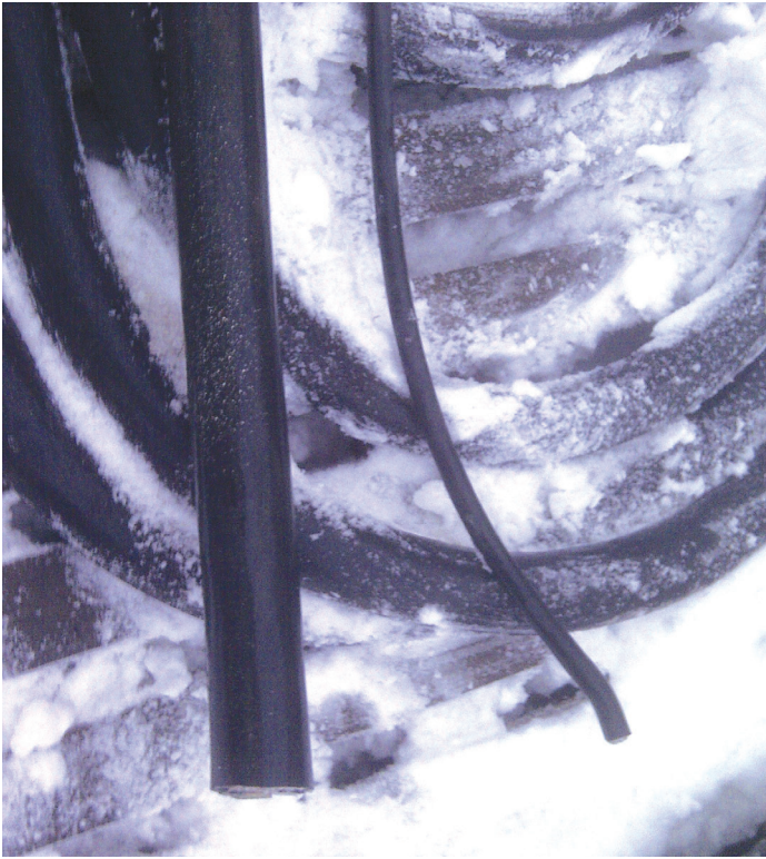
The old DLO cable, pictured left, is significantly larger and heavier than the new G-GC cable to the right.
