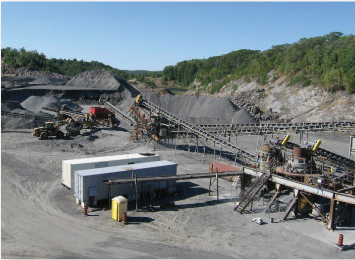
The control trailer and generator trailer at Fowler Construction's mobile crushing plant are tethered together by 200 ft of DLO cable.
