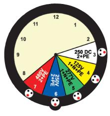
**Ground Pin location** is specified for the female connector referenced to the hour positions on the face of a clock.
