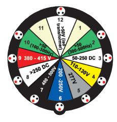
Color Slices represent Voltages 4 Wires: 3+PE
