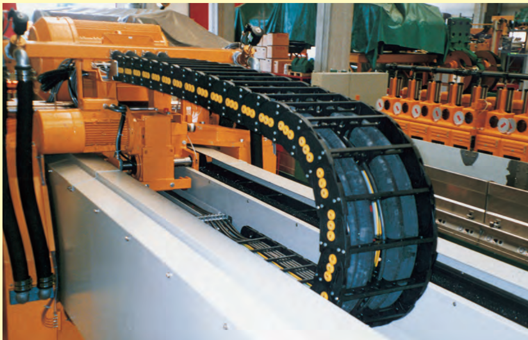
Nylon chain, type 310, in a self-supporting state.
