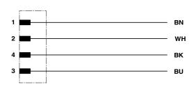
S/A cable: M12 connector on free conductor end
