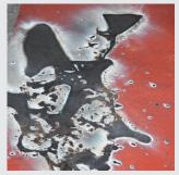
The heavy coating of our proprietary iron oxide red silicone compound sheds molten metal splashes immediately, so very little heat transfer occurs.
