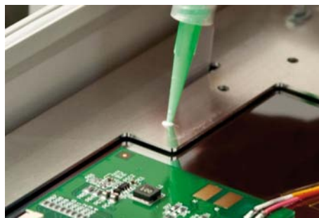
The installation process efficiently compensates for dimensional and processing tolerances, and also for the effects of thermal expansion or mechanical loads such as vibrations.
