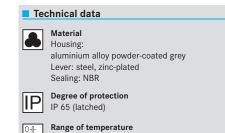
$-40^{\circ}\text{C}$  - + 100°C, temporary up to +125°C
