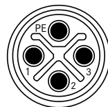
3+PE-pos. S-coded for power supply
