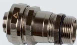
ISO cable-hose fitting, compact, male, nickel plated brass, double seal according EN 45545-2, HL1 / HL2 / HL 3, table R22 and R23 (incl. connection set).
