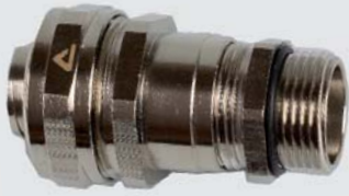
ISO cable-hose fitting, compact, male, double seal acc. EN 45545-2, HL1 / HL2 / HL 3, table R22 and R23. (incl. brass connection set).
