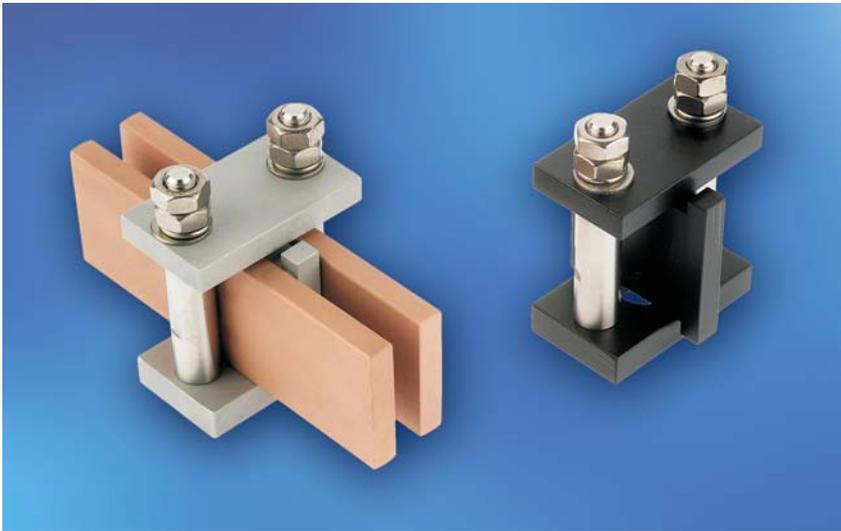
Busbar supports for use as **sliding** support for long busbars which must slide in the holder to allow the thermal expansion. By using this design the lower part of the holder is fastened to the support by means of the stay bolts prior to assembly. Now a simple insertion of the busbars between the stay bolts is possible and a time saving assembly is realized.
