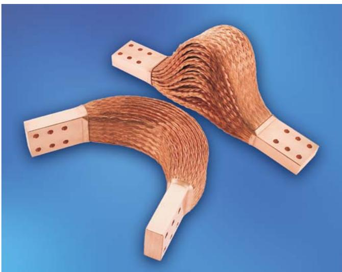
Also for applications in the field of welding machines we deliver flexible braided high current connectors to realize movements in two as well as three dimensions. They consist out of several layers braided copper tapes, similar to the welding gun designs, but with a contact area width up to 120 mm or greater and conductor cross-sections up to 4000 mm<sup>2</sup>.
