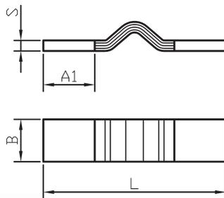
Expansion connectors in standard design. The width and the thickness of the contact areas are in coordination with the usual dimensions of the traditional busbar systems. With drilling on request, e.g. according to DIN 43673 page 1 +2, DIN 46206 page 2 or according to your drawings/samples or wishes. On request it is also possible to deliver expansion connectors with other dimensions or in bended design according to your drawings as well as with coated contact areas (e.g. tinned or silvered).
