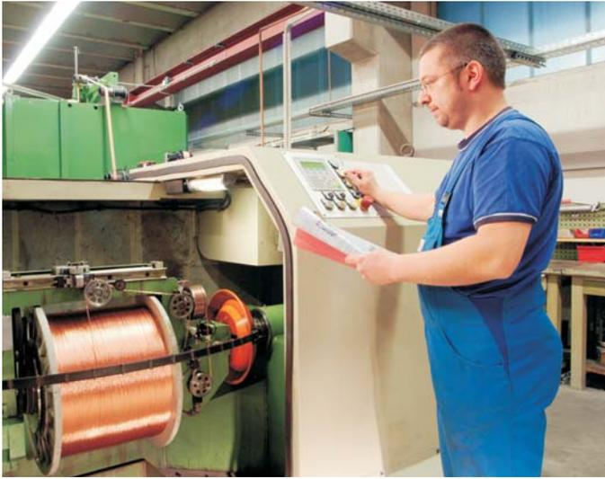
Twisting of conductors and manufacturing of round stranded cables
