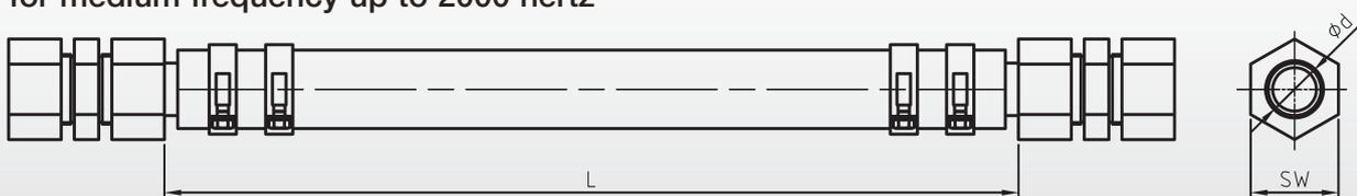
Design with pipe connections on both sides
