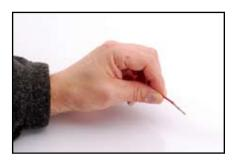
1. Grasp crimped contact approx. one inch behind the contact barrel.
