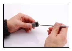
1. Remove wedge by inserting a hook into an opening of the wedge.
