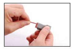
Push contact straight into receptacle until a 'click' is felt. A slight tug will confirm placement.
