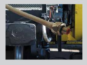
**Material:** Counter nut, body, clamping ring and ferrule are nickel plated brass with exception of size 3/8" till 1" where the ferrule is from galvanised steel. Inserts are made from PA6 (red for ISO metric, blue for Pg and white for NPT).
