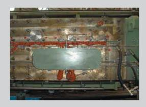
good temperature reduction and withstands molten splash. **Temperature:** -55 °C till +260 °C continuous. Under flame till +800 °C for approx. 20 minutes. Radiation heat till +800 °C for approx. 20 minutes. Molten metal splash till +1640 °C for 15-30 seconds. **Colour:** Red, other colours available on demand.
