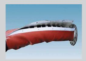
Cover specifications: Iron-oxide silicon rubber, excellent oil resistant, halogen-free, good short term flame protection, good temperature reduction, withstands molten splash. Hiproblanket Wrap H-TB enables a finished assembly to be certified to MIL-I-24244, ASTM E84.84A, ASTM E162.
