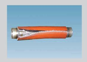
oil resistant, halogen-free, good short term flame protection, good temperature reduction, withstands molten splash. Hiproblanket Wrap H enables a finished assembly to be certified to MIL-I-24244, ASTM E84.84A, ASTM E162.
