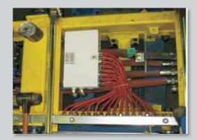
Material: Counter nut, body, clamping ring and ferrule are nickel plated brass with exception of size 3/8" till 1" where the ferrule is from galvanised steel. Inserts are made from PA6 (red for ISO metric, blue for Pg and white for NPT).
