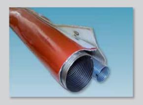
Cover specifications: Iron-oxide silicon rubber, excellent oil resistant, halogen-free, good short term flame protection, good temperature reduction, withstands molten splash. Hiproblanket Wrap H-TB enables a finished assembly to be certified to MIL-I-24244, ASTM E84.84A, ASTM E162. Weight material: 3,26 Kg/m2
