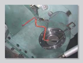
**Temperature:** -55 °C till +260 °C continuous. Under flame till +538 °C for approx. 20 minutes. Radiation heat till +538 °C for approx. 20 minutes. Small molten metal splash till +1200 °C for 15-30 seconds. **Colour:** Red.
