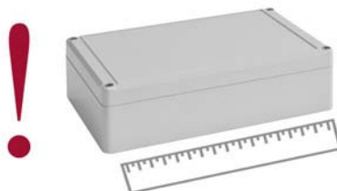
Material shrinkage may result in ABS enclosures being approx. 0.1 - 0.25% larger
