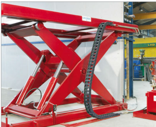
UNIFLEX Series cable and hose carriers on a scissored coil lift
