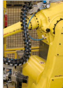
ROBOTRAX cable carriers on an assembling system Photographs: Gerstung Systemtechnik GmbH
