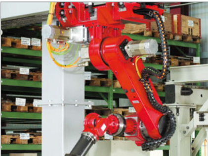
ROBOTRAX cable carrier system on a combined portal and buckling arm robot application Photographs: Güdel AG, Langenthal
