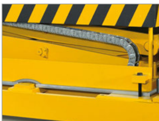
Steel cable carriers on a scissored coil lift Photographs: SÜDO GmbH
