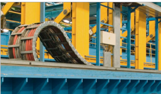
Steel cable carriers on a laser cutting machine
