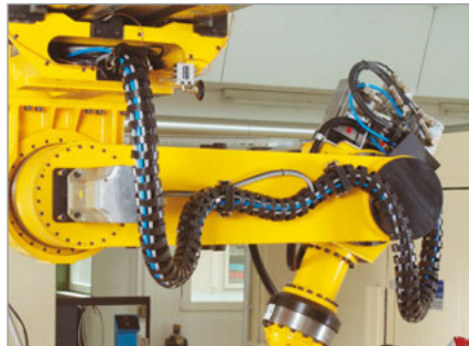
ROBOTRAX cable carrier system on a combined portal and buckling arm robot application Photographs: Güdel AG, Langenthal
