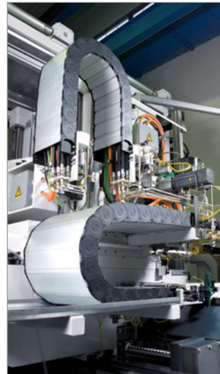
Cable and hose carriers of the MASTER LT series on a tube end processing machine
