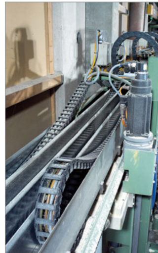
MONO Series cable and hose carriers on a wood processing machine
