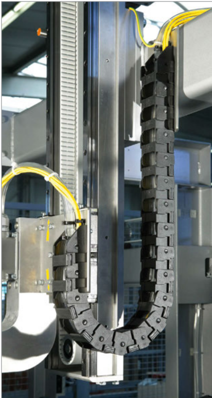
MONO and UNIFLEX Series cable carriers on packaging machines Photographs: Transnova-Ruf GmbH
