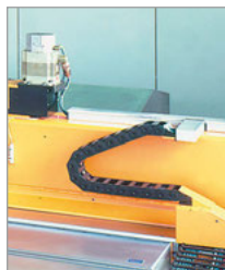
UNIFLEX Series cable carrier and KABELSCHLEPP telescopic cover on a highspeed machining center
