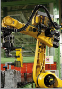
ROBOTRAX cable carriers on a jointed-arm robot Photographs: Daimler Chrysler AG
