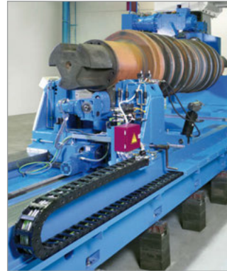
Cable and hose carriers of the UNIFLEX and MONO series on a roll neck milling machine
