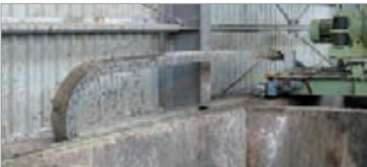
Steel cable carriers with steel band cover on a shredding system Photographs: Lindenschmidt KG
