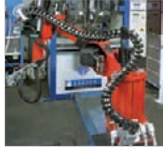
ROBOTRAX cable carrier system: Angle of rotation about 180° without channel system on a buckling arm robot application Photographs: Reis Robotics, Arthur Bräuer GmbH & Co. KG
