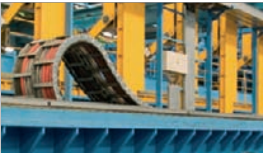
Steel cable carriers on a laser cutting machine Photographs: Meyer Werft GmbH
