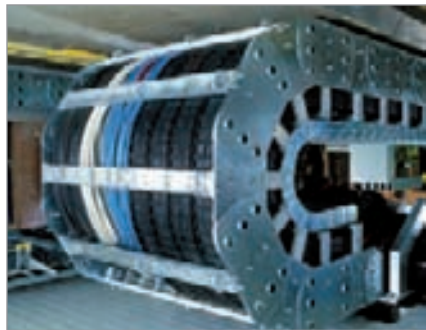
Type MK 0475 cable carrier for separating the cables in a steel cable carrier system, Type 3200 on the ZEUS detector
