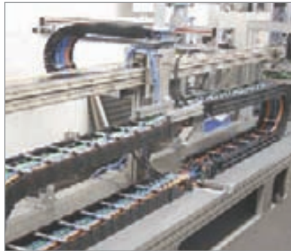
■ High-speed test stand ■ Durability tests exceeding 25 million cycles
