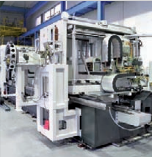
Cable and hose carriers of the MASTER LT series on a tube end processing machine Photographs: Rottler Werkzeugmaschinen GmbH
