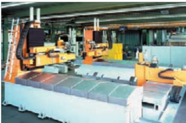
UNIFLEX Series cable carrier and KABELSCHLEPP telescopic cover on a highspeed machining center Photograph: EiMa Maschinenbau GmbH
