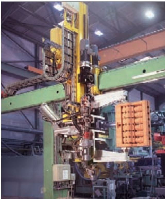
ROBOTRAX cable carrier system and steel cable carriers on a manipulator for handling crankcase core stackings Photographs: Hottinger Maschinenbau GmbH
