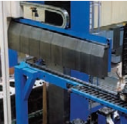
■ Cross-beam cover at a milling machine
