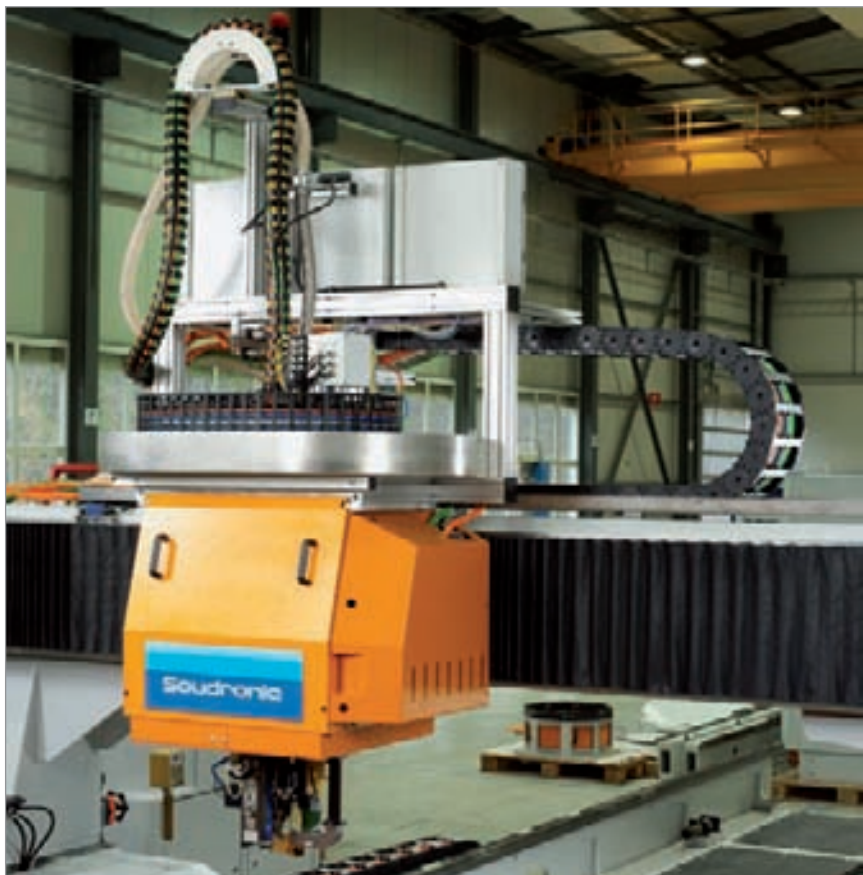
ROBOTRAX, K Series and M Series cable carriers on a laser cutting machine Photograph: Soudronic AG Automotive
