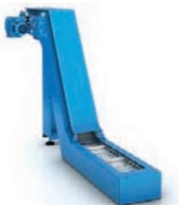
■ Straight/rising/straight design Max. incline 60°
