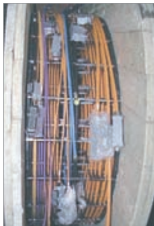
■ 125 m travel length: carrier fully harnessed with LIFE-LINE Series 700
