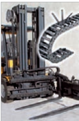
UNIFLEX Series cable and hose carriers on a forklift Photograph: Ing. G+M Schurz GesmbH
