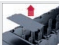
Detach the cover from the chain link
