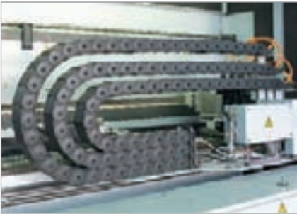
UNIFLEX Series cable and hose carriers on an automatic wood processing machine Photographs: Homag Holzbearbeitungssysteme AG
