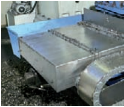
■ Telescopic cover at a milling machine
