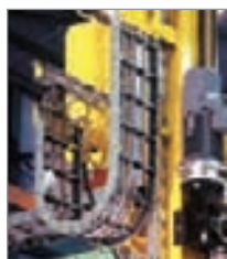
ROBOTRAX cable carrier system and steel cable carriers on a manipulator for handling crankcase core stackings Photographs: Hottinger Maschinenbau GmbH
