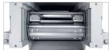
Replacement of individual hinge belt plates at the discharge
