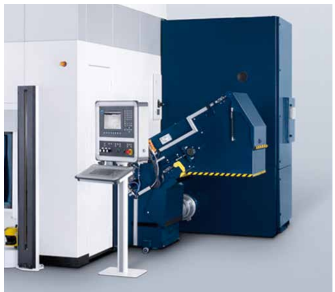
WAVE-BELT conveyor on a laser cutting machine
