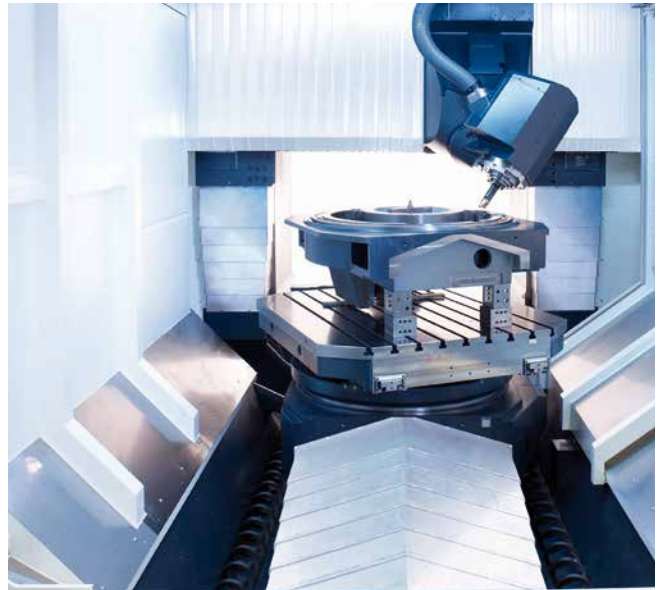
Telescopic cover with harness mechanism on a 5-Axis portal milling machine
