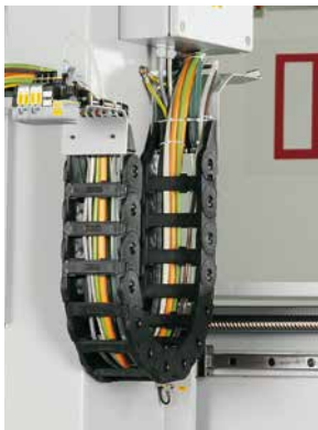
Plastic cable carrier on a CNC-machining center. Photographs: Reichenbacher GmbH
