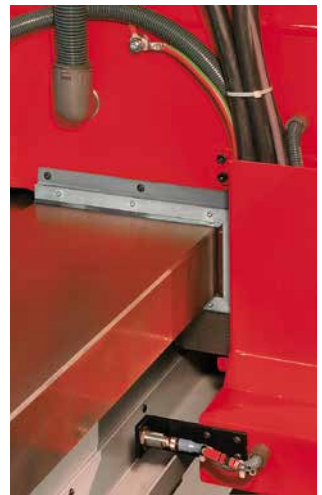
Telescopic cover with harness mechanism on a 5-Axis portal milling machine
