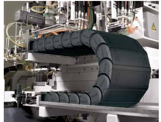
Cable carrier system TKA Series on a machining center
