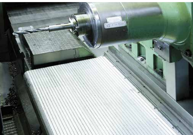
Link apron cover on a milling machine
