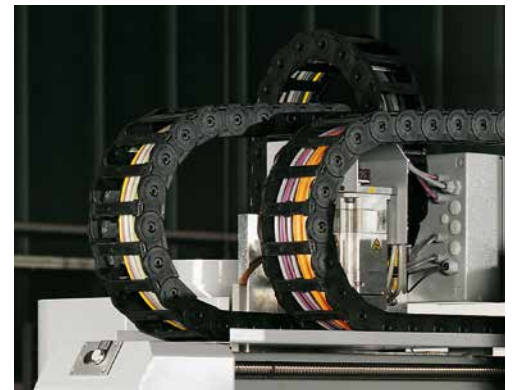
Cable carrier system TKA Series on a machining center
