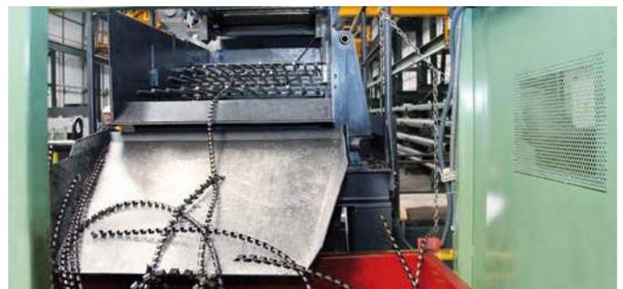
Lange Späne fallen in einen separaten Container. Long chips are dropped into a separate container.
