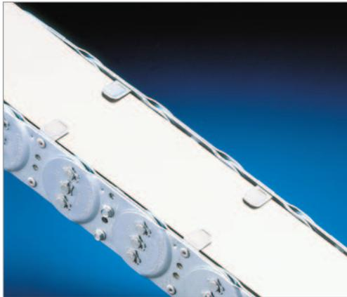
Steel strip covers made of rust and acid resistant spring steel strip can be supplied for protection of the cables against flying sparks, radiant heat and small chips. **Note:** Only applicable with horizontal single cable carrier (within the radius of curvature, no reverse bending).
