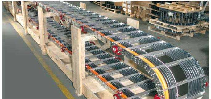
■ Ready-to-connect assembled plastic cable carrier system, packed ready for installation
