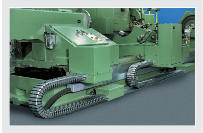
CONDUFLEX cable carrier tubes on a roll grinding machine.
