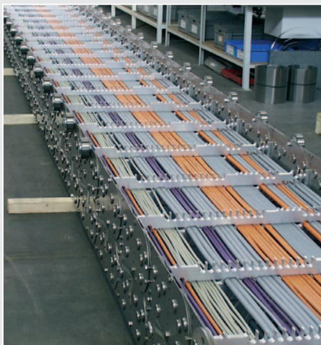
Steel cable carriers with TRAXLINE Cables for Motion.
