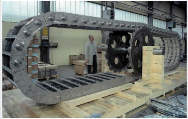
Steel cable carrier with load-bearing bolts.
