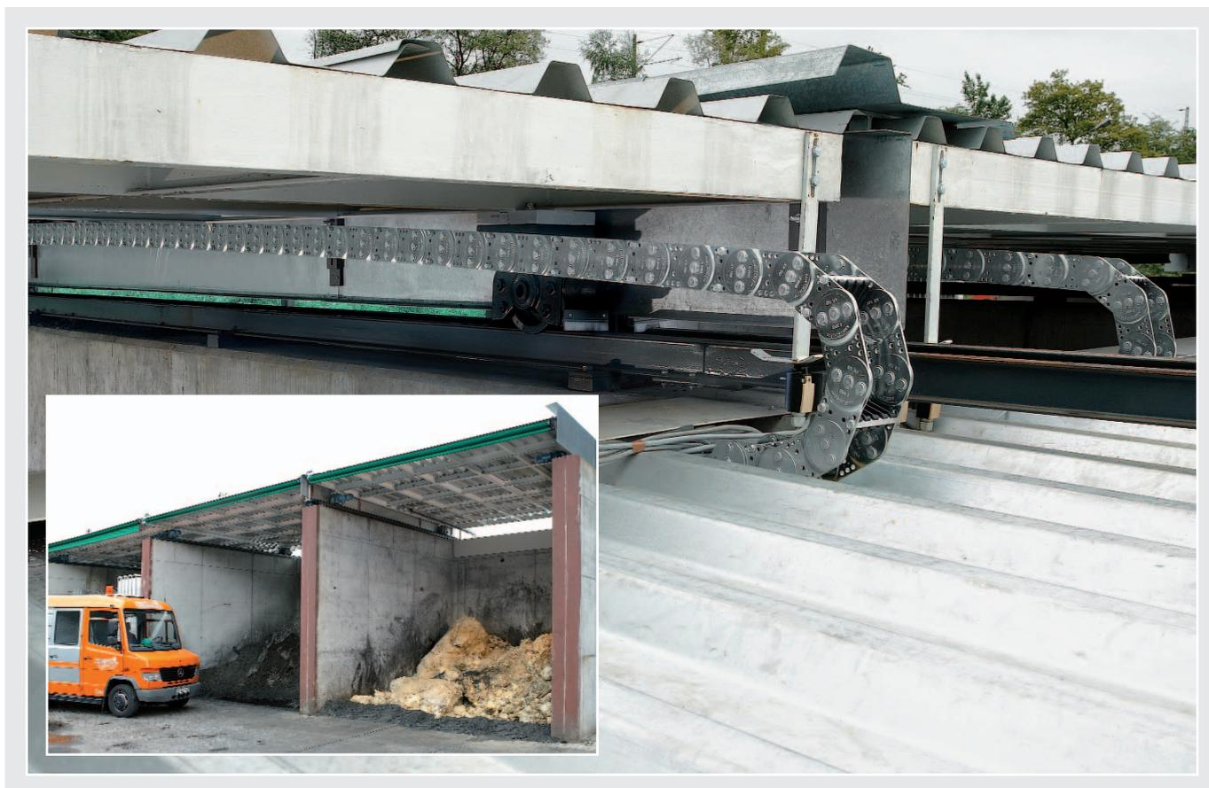
Steel cable carriers on a movable roof construction. Photographs: Lindenschmidt KG
