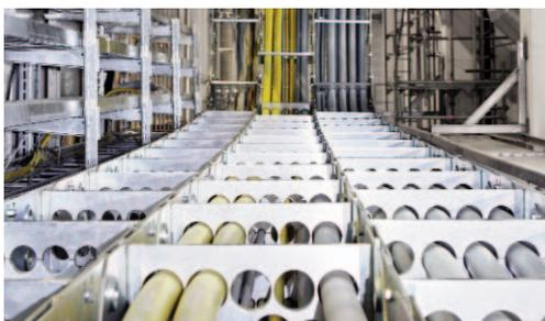
If the available space will not allow a cable carrier system to be installed because of the required width, a **nesting** or **opposing** system can be arranged.
